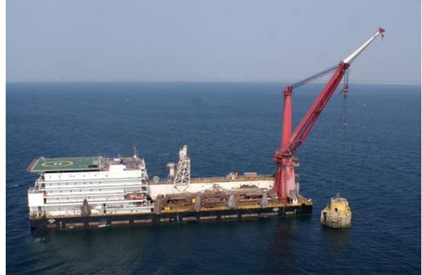
Salvage, refurbishment and reinstallation of SPM buoy
