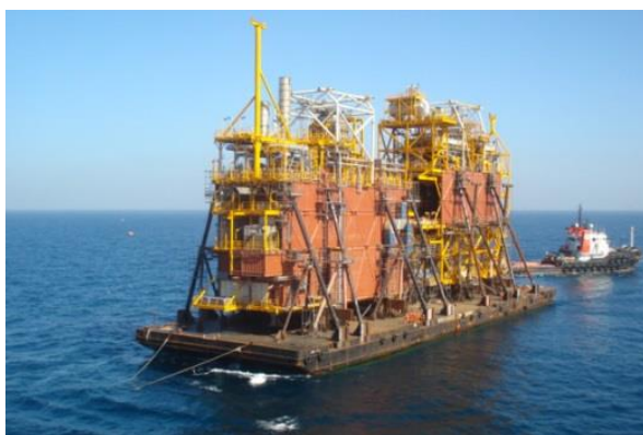
Marine towage approval of offshore structure
