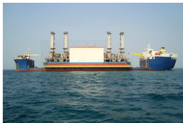
Float-on and float-off operation for complex marine transportation
